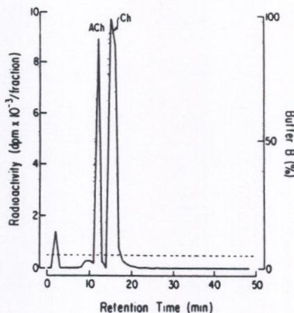
FIG. 5. Isocratic separation of [ $^{14}\text{C}$ ]acetylcholine and [ $^3\text{H}$ ]choline standards. A mix of [ $^{14}\text{C}$ ]acetylcholine (ACh) and [ $^3\text{H}$ ]choline (Ch) standards was separated utilizing a mixture of 95% buffer A and 5% buffer B. Other details of the chromatographic conditions, including buffer composition are described in the legend to Fig. 1 and under Materials and Methods.
